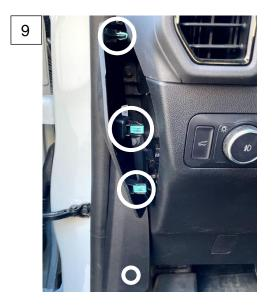
Carefully pull the edges of the headlight control dash panel until the clips release. Remove the arrowed headlight control unit connector.
