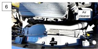
7. Remove the circled connector on the air cleaner cover and the two arrowed clips attaching the harness. Using a flathead screwdriver, remove the intake air boot clamp. Pull up on the air cleaner box to remove and set aside.
